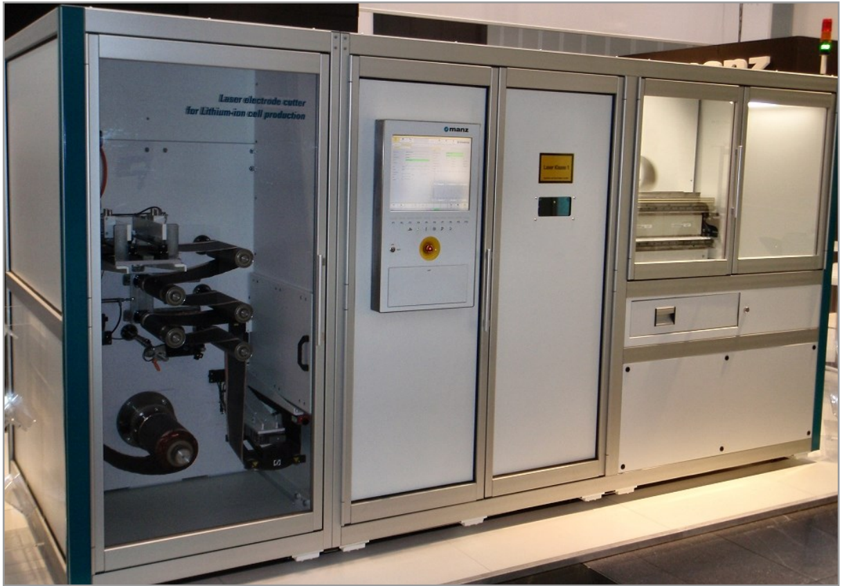
Abb. 10 - Laser electrode cutter for Lithium-ion cell production. Bild: Torsten Pörschke
